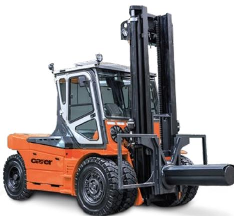
This forklift truck is the maximum expression of the force and power of Carer's standard range of forklift trucks. It can handle loads weighing up to 16,000 kg.
