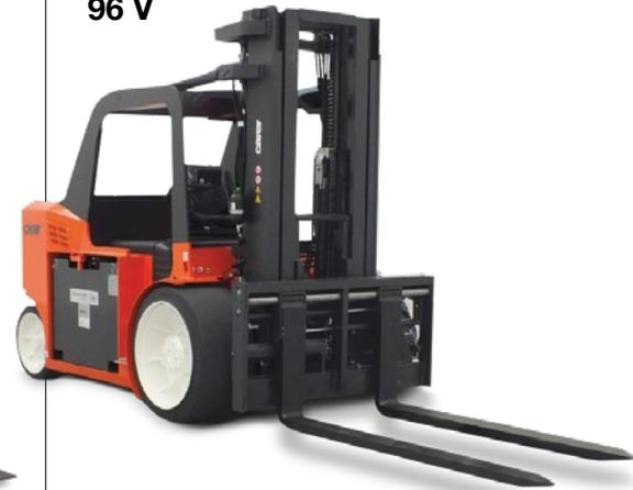
Specifically designed with cushion and Vulkollan tyres to ensure a maximum capacity up to 16,000 kg. Thanks to its extremely compact sturdy frame, this forklift truck is the ideal solution to handle heavy loads in closed and narrow spaces, ensuring an extremely small steering radius.
