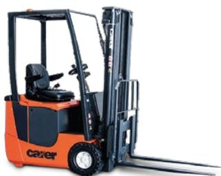
Overall width 85 cm, voltage 48 V, front-wheel drive with 2 AC motors, electric steering, oil bath brakes: these are some of the features that make the N 08-10 the most advanced forklift truck in his class. Power, high performance, easy handling and comfort make it ideal for intensive work shift in narrow and limited space.
