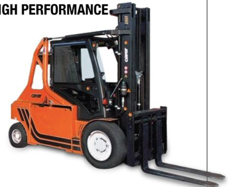
Designed to withstand long operating time at very high performance levels, F 60-100 HD<sup>2</sup> (Heavy Duty) can be considered the highest expression of the principles and technology developed by Carer over the years. Thanks to the super steer axle, the electronic differential, the noticeable compact design of the forklift truck and maximum comfort of the driver's seat, the F 60-100 HD<sup>2</sup> is the right forklift truck for particularly heavy duty applications.
