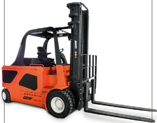
The driver's seat is wide and spacious. Controls and instruments are arranged respecting ergonomic sizing requirements. The steering wheel has a tilting steering column and can also be adjusted depth-wise. Exceptional visibility at the front and the back thanks to the raised driving position. The electronic control ensures maximum silence and maximum motor performance.
