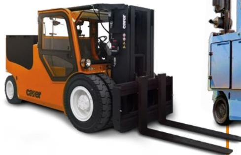
Designed to handle extremely heavy loads in containers, the K 100-120 H provides high performance levels and wide manoeuvrability thanks to a set of cameras that ensure maximum visibility at the rear during challenging handling manoeuvres. The K 120 H is the only forklift truck with a compact size and 12,000 kg capacity that can operate inside a container.
